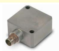
The DC response accelerometers are gas & Oil damped, resulting in minimal influence of thermal changes. These low-impedance units operate with a supply voltage from 8 to 24 V DC, and a supply current of 5 mA. The ±2 volt differential output is DC-coupled at a bias voltage of 2.5 V DC, and a 2.5 V reference is built-in for differential measurements. The units can be used with either differential or single-ended input.
